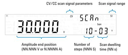
4 After configuring the scan signal parameters, press **Shift > Save** to save, and **Shift > Exit** to exit the utility menu.
