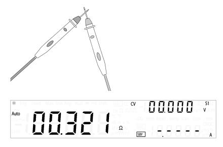
**4** Press **Null** to enable the null function.
