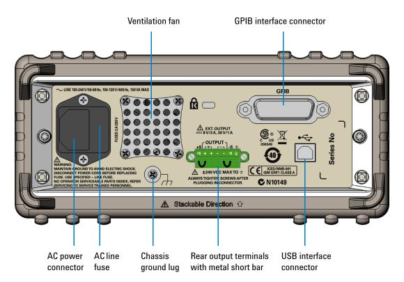
Connect the power cord to the AC power connector. The mains plug should only be inserted in a socket outlet that provides protective earth contact.
