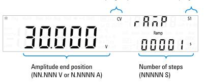
CV/CC ramp signal parameters Ramp signal range
